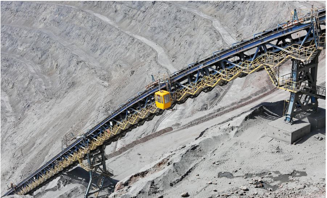
Fig. 2. Steeply inclined conveyor at the Muruntau gold pit
