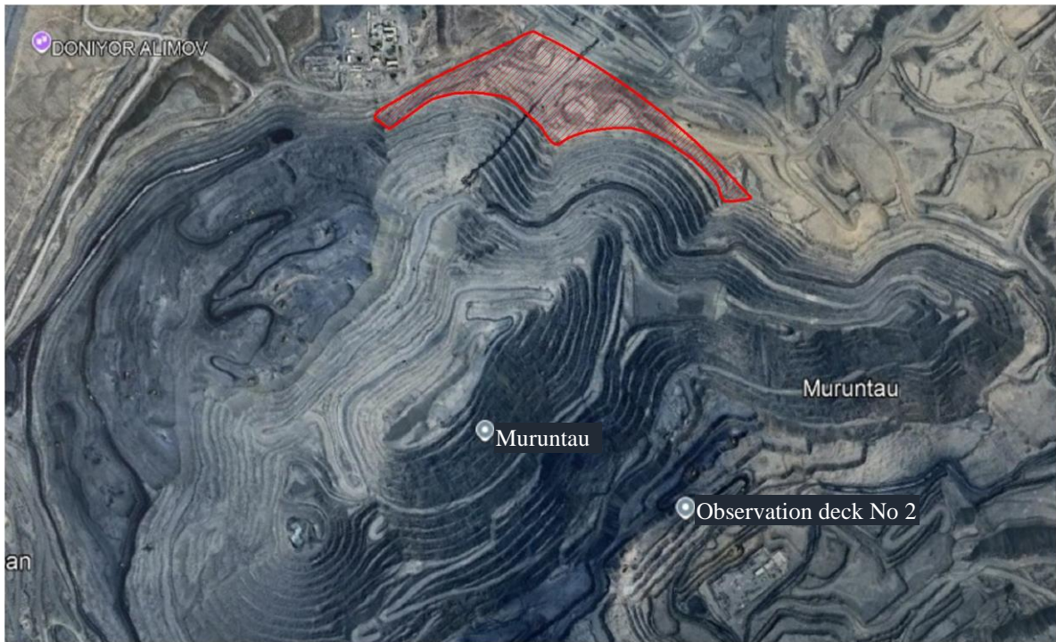
Fig. 3. The general plan of the Muruntau gold pit with a preserved ore block highlighted
